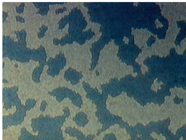
Figure 5. Optical texture of compound 3 obtained 2 K above the clearing temperature by application of an electric field of 25 \text{ V } \mu\text{m}^{-1} . One polarizer is rotated by +5^\circ from the crossed position.
