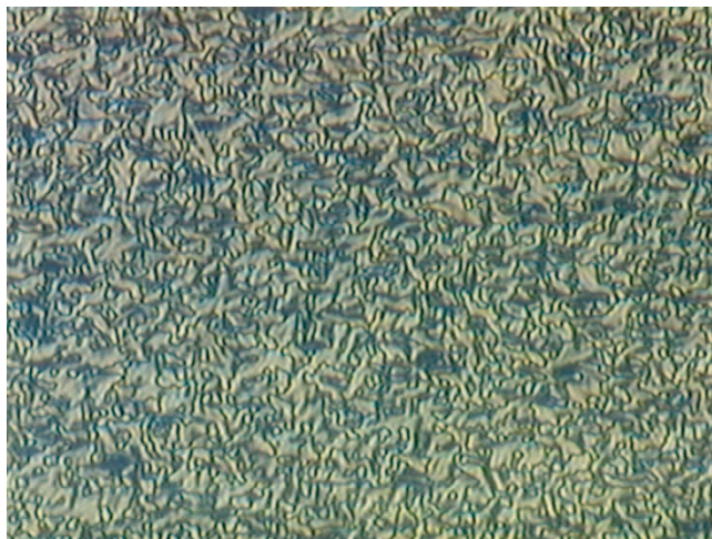
Figure 3. Fan-like texture obtained after removing the applied electric field (compound 3 , 180°C).
